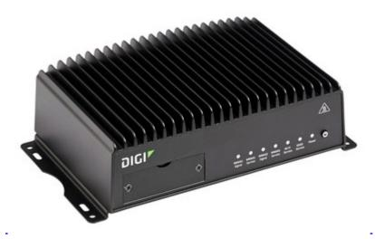
Digi International has optimized its <u>Digi TX54</u> LTE router product line to use AWC's patented AW12 USB LTE Modem, which is FirstNet Ready<sup>™</sup>, to enhance data throughput and connectivity. FirstNet Ready<sup>™</sup> devices support access to the dedicated FirstNet network core, First Priority® on FirstNet– which includes *always-on* priority and preemption for first responders – and the Band 14 spectrum.
